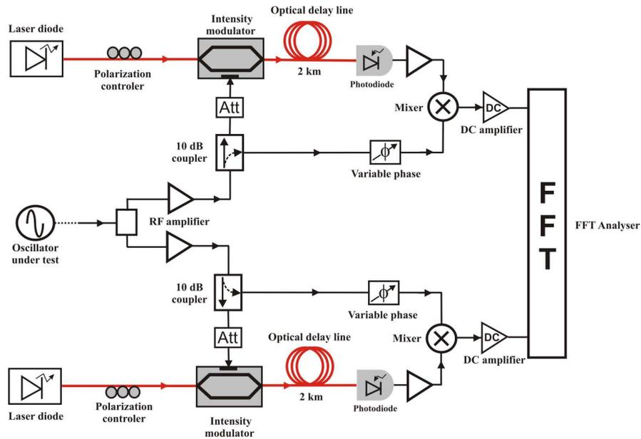
Fig. 1. Principle of the phase noise measurement bench system using a double optical delay line.
