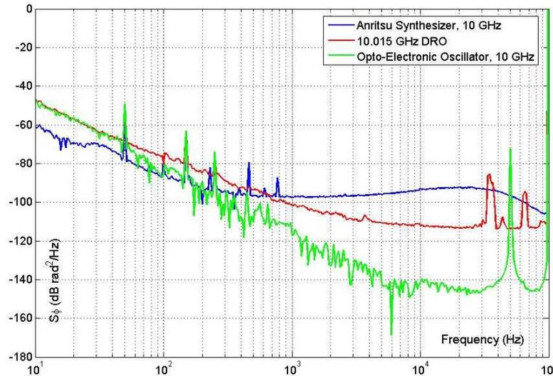
Fig. 2. Phase noise measurement in X-band of an Anritsu microwave synthesizer, a DRO and an optoelectronic oscillator.
