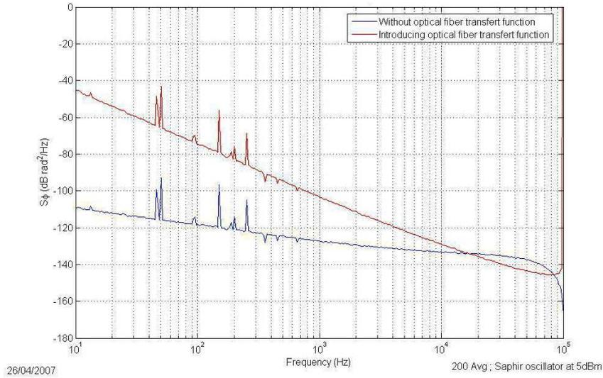
Fig. 3. Phase noise measurement of a sapphire oscillator.
