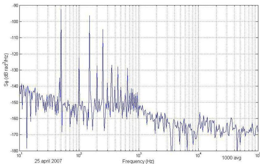
Fig. 4. Phase noise floor of the bench measured with sapphire oscillator.
