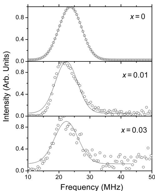
Fig. 4. Normalised  $^{139}\text{La}$  NMR spin-echo spectra for  $(\text{La}_{0.67}\text{Ca}_{0.33})(\text{Mn}_{1-x}\text{Sn}_x)\text{O}_{2.94}$  with  $x = 0, 0.01$ , and  $0.03$  at 4.2 K. Solid lines denote the Gaussian fits to the spectra.
