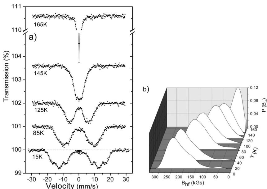
Fig. 1. (a) Temperature variation of the selected  $(\text{La}_{0.67}\text{Ca}_{0.33})(\text{Mn}_{0.97}\text{Sn}_{0.03})\text{O}_{2.94}$  Mössbauer spectra. Solid lines denote the best fits and small black area (at 15 K spectrum) denotes the fitted contribution of the paramagnetic impurity phase. The base lines of the  $T > 15$  K spectra are arbitrarily off-set. (b) Temperature dependence of  $P(B_{\text{hf}})$  obtained from the Mössbauer spectra.
