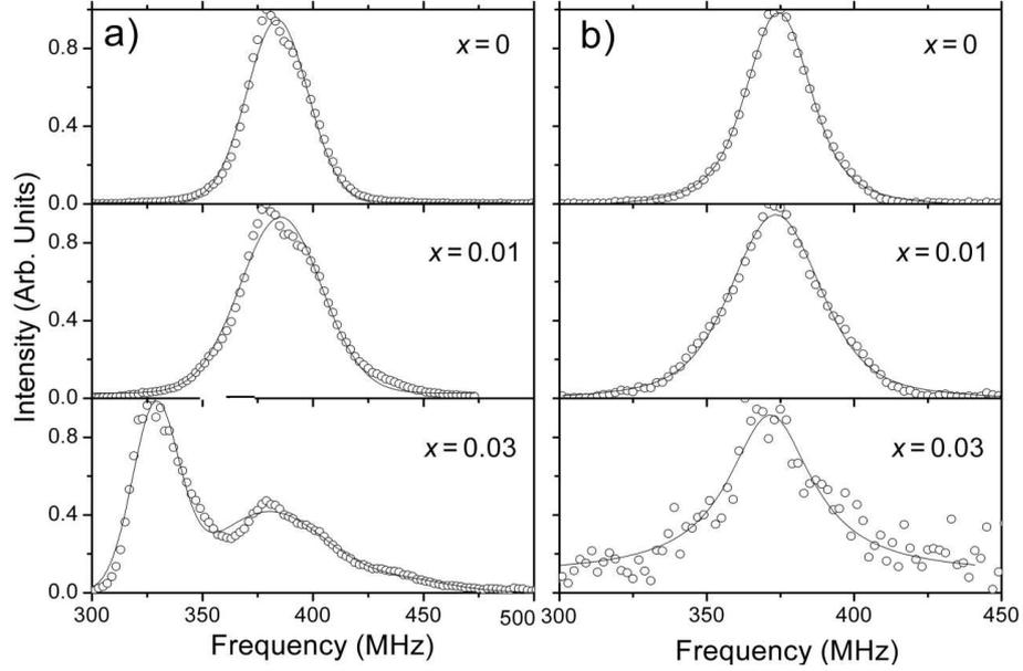
Fig. 3. Normalised  $^{55}\text{Mn}$  NMR spin-echo spectra for  $(\text{La}_{0.67}\text{Ca}_{0.33})(\text{Mn}_{1-x}\text{Sn}_x)\text{O}_{2.94}$  with  $x = 0, 0.01,$  and  $0.03$  at  $4.2\text{ K}$  (a) and  $77\text{ K}$  (b). Solid lines denote the single or multicomponent Gaussian fits to the spectra.
