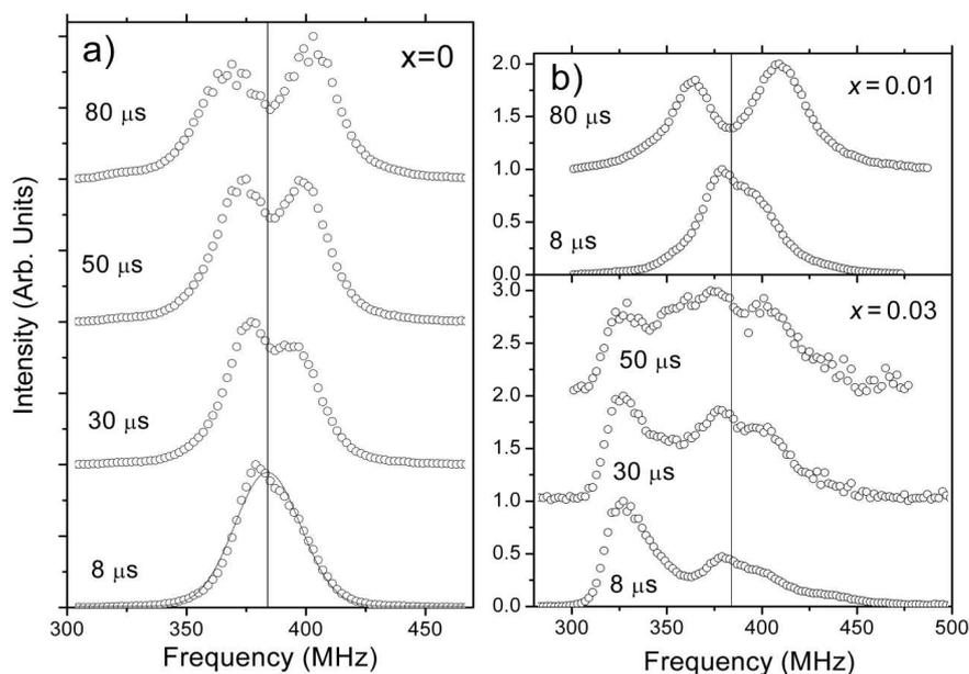
Fig. 5. Pulse-spacing ( $\tau$ ) dependence of the normalised  $^{55}\text{Mn}$  NMR spin-echo spectra for  $(\text{La}_{0.67}\text{Ca}_{0.33})(\text{Mn}_{1-x}\text{Sn}_x)\text{O}_{2.94}$  with  $x = 0$  (a), and  $x = 0.01, 0.03$  (b), at 4.2 K. Solid line denotes the Gaussian fit to the  $x = 0$  spectrum with  $\tau = 8 \mu\text{s}$ .
