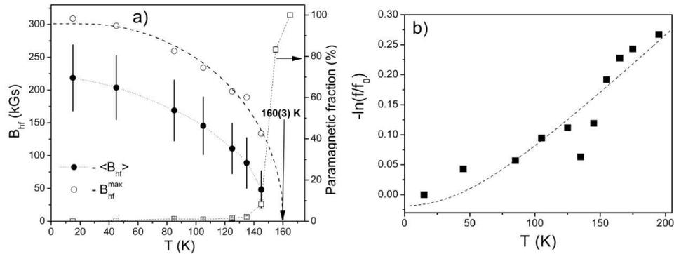
Fig. 2. (a) Temperature dependence of  $\langle B_{hf} \rangle$  (full circles),  $B_{hf}^{max}$  (open circles),  $\sigma$  (vertical lines around  $\langle B_{hf} \rangle$  values) and paramagnetic fraction (open squares) obtained from  $(La_{0.67}Ca_{0.33})(Mn_{0.97}Sn_{0.03})O_{2.94}$  Mössbauer spectra. The meaning of dashed line is explained in the text. (b) Temperature variation of the  $-\ln(f/f_0)$  parameter. The meaning of dashed line is explained in the text.
